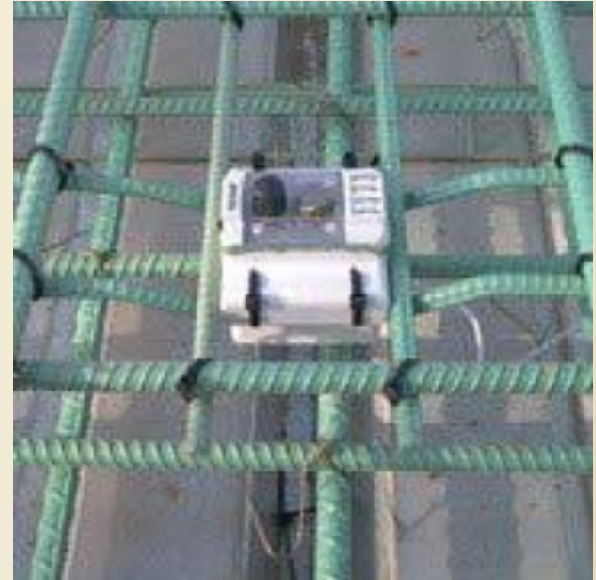
Embedded Corrosion Instrument
